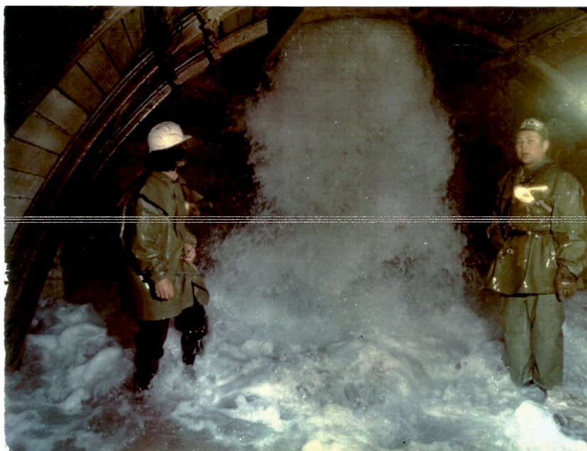
Fig. 2 Water inrush from ore bearing dolomites ca. 1.0 \text{ m}^3/\text{s} (Photo by J. Leśniak)
